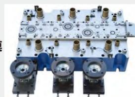
**D110mm压缩机电机三列自扣级进模**
